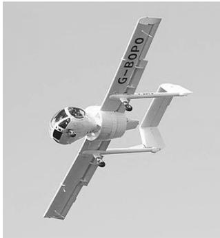
Back in December 1979 one of the weirdest looking aircraft yet seen was to take to the sky. Because of its odd appearance, with its prominent perspex cabin, it was nicknamed “Bug Eye”. It was designed to provide excellent visibility and to have the low speed capability of a helicopter but at a much lower cost and with the advantage of being as easy to fly as a conventional light aircraft.
